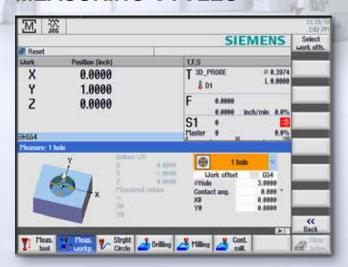
Several standard cycles are available to find centers of holes, part edges, and bosses. Cycles can also be used to measure finished parts and display the reading.
