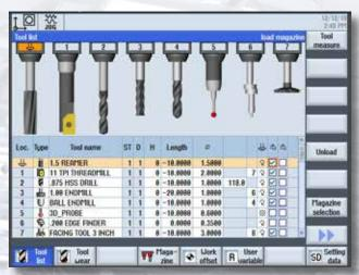
Graphic display shows the type and name of the tool. You can also control spindle direction and coolant. Tool life monitoring is also standard for time in cut or part count.
